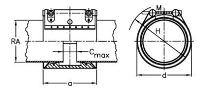
a = 142 Weight a piece = 6.1 C max with insertion band = 35 d = 230
